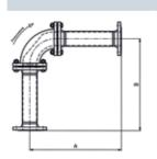
Connector Pipes for Master-Protect Pipe-Bends
