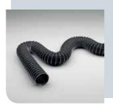
Suction & Blower hose made from VITONcoated polyester fabric, for corrosive media up to +210 °C, electroconductive ≤ 10<sup>4</sup> Ohm
